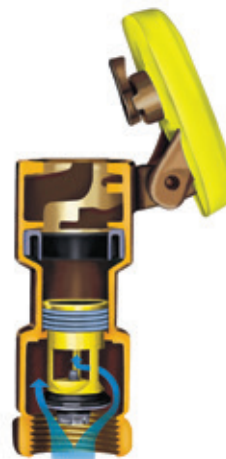
Quick-Coupling Valve Cutaway
